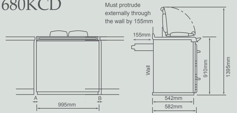
\* Flue shown above is for 680KCD C/F model only, which uses a condensing flue.
